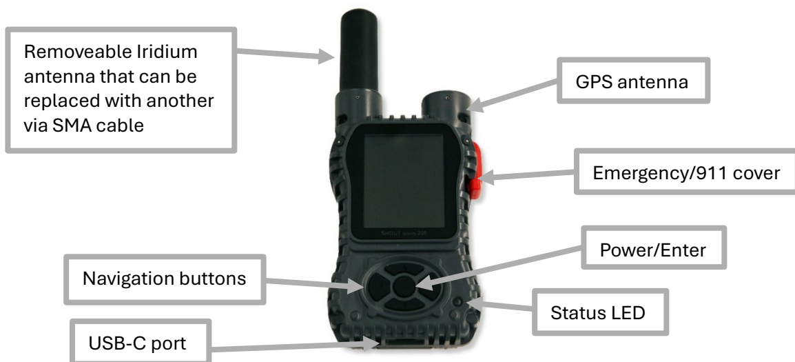
Figure 1: SHOUT nano 200 external components
