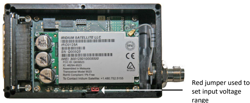
Figure 2: Power Input Setting for the A3LA-RM
