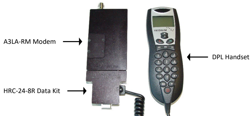
Figure 3: A3LA-RM Connected to a DPL Handset via the HRC-24-8R
